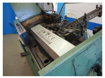
Mule's engineered Retrofit Kits convert existing thread rolling equipment into high-precision machines with the ability to create, save and accurately repeat die setups quickly. This new technology allows fastener manufacturers to capture the intrinsic knowledge of their most valuable workers and repeat setups in a fraction of the time and with the same exacting control.
